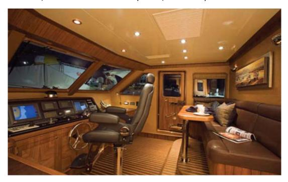
The helm is a simple fiberglass console with duplicates of the monitors and controls in the pilothouse. A Stidd chair and built-in double seat provide a fine view over the bow, and there is a large flat space for charts to starboard, plus recessed trays for all the stuff you need: sunglasses, cruising guides, binoculars, and more.
